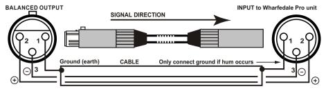
BALANCED INPUT WIRING TO WHARFEDALE PRO UNIT WITH 1/4" JACK to XLR CONNECTORS
